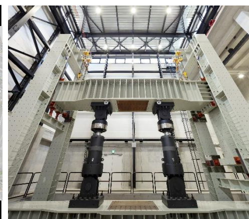
Photo.4 The large-scale seismic loading system Taisei Corporation
